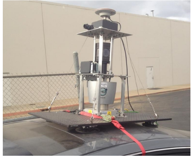
Fig. 3: Navigation and Mapping sensor platform. Equipped with GPS/INS unit, monocular camera, 360 degree camera, 2D LIDAR, RADAR, and Velodyne LIDAR.
