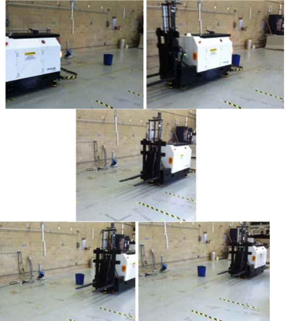
Figure 6: (top-left to bottom-right) Series of snapshots showing the AGV performing obstacle detection and avoidance using the spline method.
